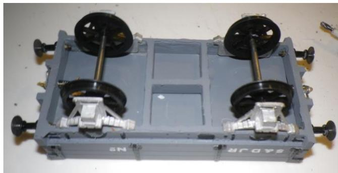
6. Repeat for the other wheel set. Use a straight edge across the back of the wheels to aid getting these parallel and square to the chassis. Then fit the axle boxes and springs (part 8)
