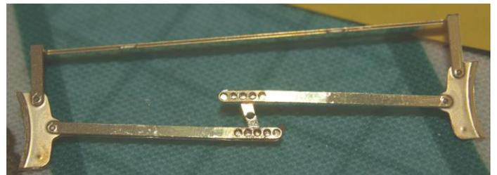
9. Fit the brake 'V' hangers (Part 12) to the sole bar lining them up with the brakes.
