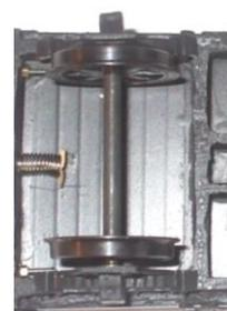
6. Assemble a wheel set, 2 x W-iron's (part 10), 2 x bearing's and 1 x wheel/axle unit, do not glue the bearings into the W-irons at this stage. Again using two-part epoxy resin, glue the assembled wheel set onto the sole-bars so that they are square and line up with the rivets as shown on the drawing.
