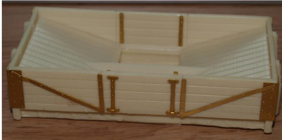
4. Next punch out the rivets on the strapping etch (part 4) and glue to the wagon as shown.
