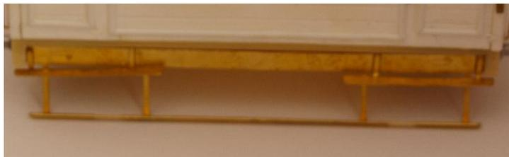
(6) Assemble the coupling hooks (part 6) and the links (part 7) then push the hooks through the hole. Next add the buffers guides (part 8) in to the holes the van ends.
