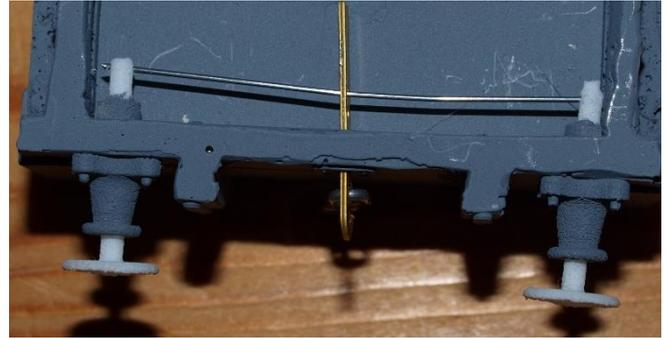
Next add the buffers heads (part 9) and spring wire (part 10). Then push the head through the holes, thread the wire into the holes on the buffer heads and the coupling hooks.
