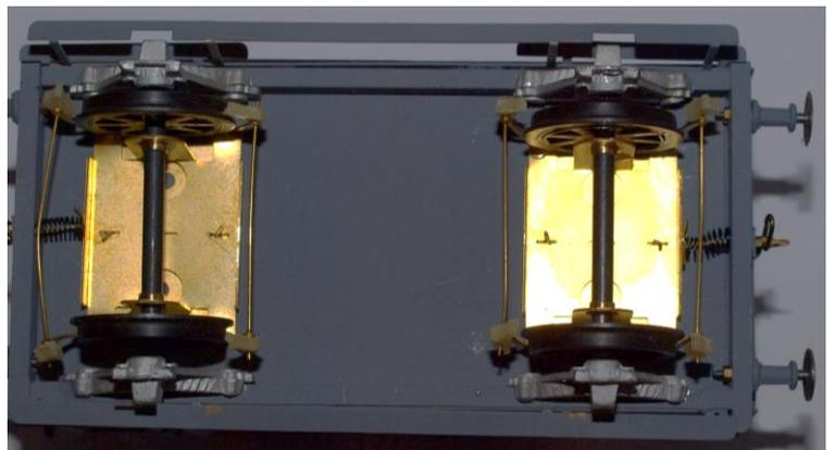
(12) Fit the cosmetic axle boxes (part 14) to the inside of the sole bars so that they line up with the wheels and the gaps in the running boards.
