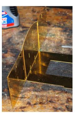
shape of the floor.. It is also a good idea to run a solder fillet down the inside of the
