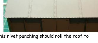
rivets in the raised banding. This rivet punching should roll the roof to its correct shape. However it may require to be rolled a little more to achieve the correct shape. Attach the roof onto the van body, being careful not to disturb the edge strips.
