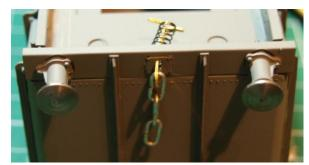
back of the coupling hook and bend the tags over to secure the spring in place. Then fix the four buffers (part 21) into the holes in the buffer beam using two part epoxy.
