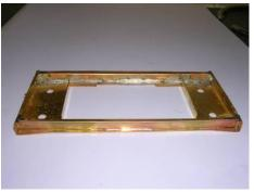
5. Next remove the buffer beam reinforcing plates (part 3) and punch out the half etched rivets and tin the back of each piece with 188C solder. Now sweat the plates onto the half etched square in the front of the buffer beam.
