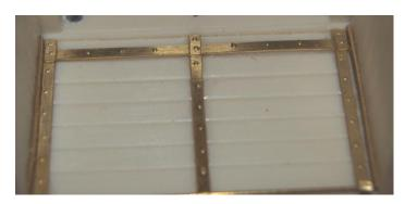
7. Fit the strapping as shown on the outside of the wagon. Note that the outside etched door is the full width of the wagon and does not have half etched tags on the top of the three uprights.
