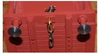
bend the tags over to secure the spring in place. Repeat for the
