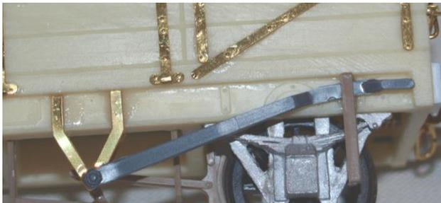
10. Fix brake lever and ratchet casting (part 13) to the outside V-hanger as shown.
