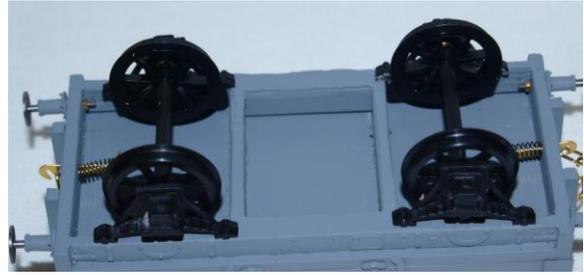
9. Glue the brake gear (part 11) onto only the one side of the wagon, as shown. Then glue the outside V-hanger (part 12), into position on the sole-bar and to the spigot of the brake gear casting.
