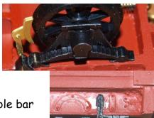
13. Fit the brake ratchet (part 11) to the sole bar as shown
