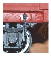
20.fit the brake ratchet (part 11) to the sole bar as shown
