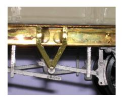
Next fix the brake lever (part 13) and ratchet casting (part 14) to the sole-bar and to the out side V-hanger as shown below.
