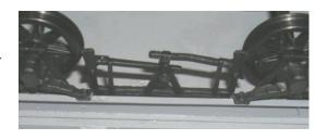
You may require to chamfer the casting so that it clears the solder filet between the chassis and the sole-bar. Glue the casting into position using two part epoxy resin; this will give you opportunity for adjustment. Position the casting with care centrally between the rivets on the sole-bar.
