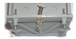
Next, assemble the links (part 9) on to the coupling hook (part 10) and push through the slot. Now push the spring (part 11) over the back of the back of
